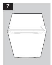
Check that the door is aligned horizontally and vertically and that the seals are closed on all sides before finally tightening the bottom hinge.
